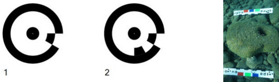
Figure 9: Coded targets used in conjunction with length and colour scale (Wreck Check Inc.) Photo on the right of a Late Bronze Age stone anchor off southern central Cyprus.
